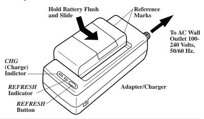
**Caution:** When a battery is attached to the adapter/charger, do not turn them upside down. The battery may fall off and be damaged or cause injury.
